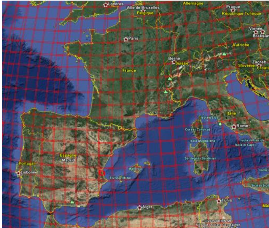
Figure 1.3: Sentinel-2X tiles, represented by red squares, over South-east Europe (image downloaded from [82]). The doubled-lines represent a 10km overlap between two consecutive tiles.
